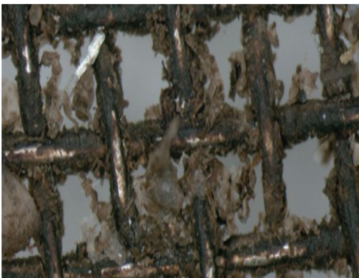
This filter screen is contaminated with particulates and a gum residue. Credit: Boeing
