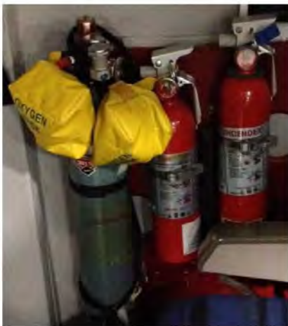
Crew/Passenger oxygen bottle with two masks; both a water and CO2 fire extinguisher is included. Also a fire ax is located in the cockpit. Location/Setup may be different according to aircraft specific.
